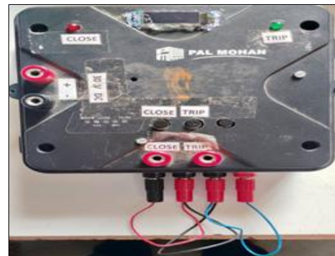
Fig 11: VCB Timing measuring meter
