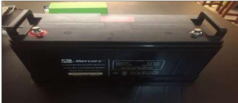
Fig 9: 12V 100AH/20HR Mercury rechargeable battery.
